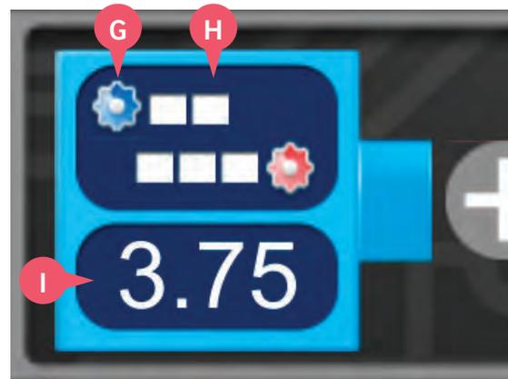
The blue gear wheel represents motor one and the red gear wheel represents motor two.
