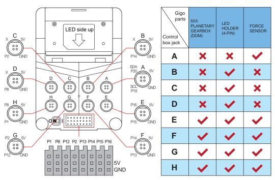
I/O pin configuration diagram (for female DuPont connectors)
