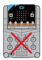
Not inserted fully into the control box.
