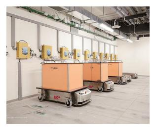
Powered Trams can run automatically and travel along a planned track on the ground. Using an infrared emitter, and infrared photoelectric crystal sensor the intensity of the reflected light determines whether the tram is on course. A controller is used to correct and adjust movement directions of the vehicle so that it can continue to run automatically on the track.
