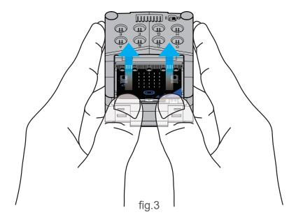
3. The micro:bit mainboard should fit flush with the sides as shown in the large picture below. If it is not, please remove it completely, ensure there are no obstructions and then try again. Make sure it is pushed in straight and not skewed.
