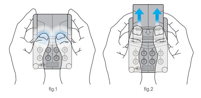
2. With the micro:bit LEDs facing upward (toward you and visible), slide the micro:bit mainboard into the control box slot.
